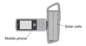
On average, the solar cells produce 0.6 joules of electrical energy each second. The solar cells have an efficiency of 0.15.
