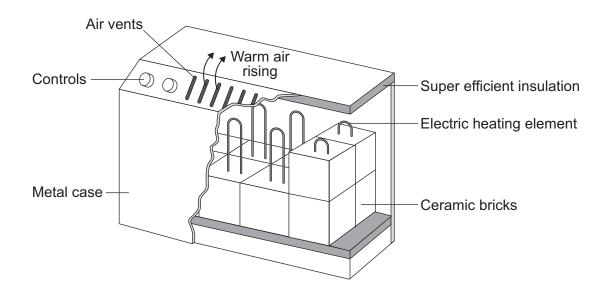
In winter, the electricity supply to a 2.6 kW storage heater is switched on each day between midnight and 7 am. Between these hours, electricity costs 5 p per kilowatt-hour.
